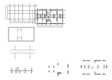
Figure 1. CAD layering divides the total information in a drawing into a number of transparent sheets, which are switched on and off, for screen viewing or printing.
