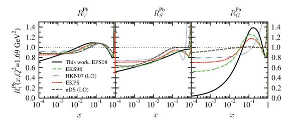
Fig. 3: Different results from leading-order (LO) QCD analyses for the ratio of the parton distribution in the lead nucleus and in the proton for valence quarks (left panel), sea quark (middle panel), and gluons (right panel) [20].
