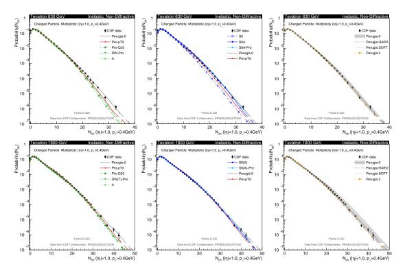
Fig. 2: Comparisons to the CDF measurements of the charged track multiplicity in minimum-bias  $p\bar{p}$  collisions at 630 GeV (top row) and at 1800 GeV (bottom row). *Left:* a representative selection of models. *Center:* different tunes of the new framework. *Right:* the range spanned by the main Perugia variations. Results with more tunes can be found at [17].
