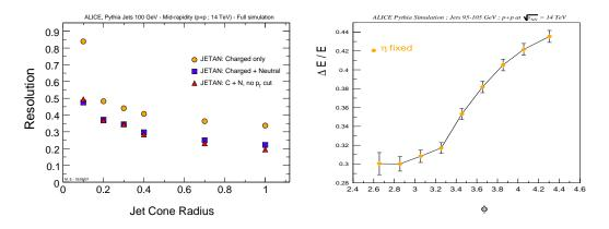
Fig. 2: <u>Left</u>: jet energy resolution of 100 GeV jets from a full ALICE simulation vs R for the three cases described in the text. Right: jet energy resolution as a function of the accepted  $\phi$  window of the center of the jet reconstructed.
