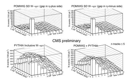
Fig. 2: Low- $\eta$  ("central slice") vs high- $\eta$  ("forward slice") HF tower multiplicity distributions for events with track multiplicity in the central tracker  $N_{\text{track}} \leq 5$ . Top left: POMWIG events with gap generated in the positive Z direction. Top right: POMWIG events with gap generated in the negative Z direction. Bottom left: PYTHIA events. Bottom right: Sum of the PYTHIA and POMWIG distributions.
