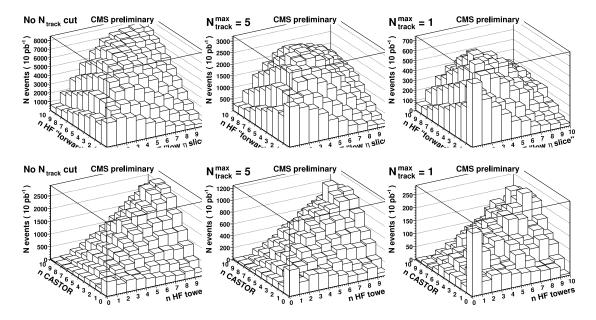
Fig. 4: HF-only (top row) and HF vs CASTOR (bottom row) multiplicity distributions for signal plus background events with no cut on the track multiplicity in the central tracker (left column),  $N_{\text{track}}^{\text{max}} = 5$  (central column) and  $N_{\text{track}}^{\text{max}} = 1$  (right column).
