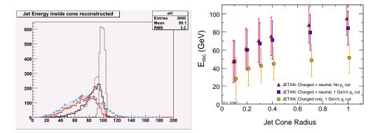
Fig. 1: Left: cone energy of 100 GeV jets reconstructed with PYCELL with R = 1 (dark dashed line), with the ALICE cone finder with detector inefficiencies and acceptance included in the simulation with R = 1 (red dashed), without detector effects but R = 0.4 (dark full), with both effects (red full). The markers shows the result from a full simulation. Right: cone energy of  $100 \pm 5$  GeV fully simulated jets vs R for the three cases described in the text.
