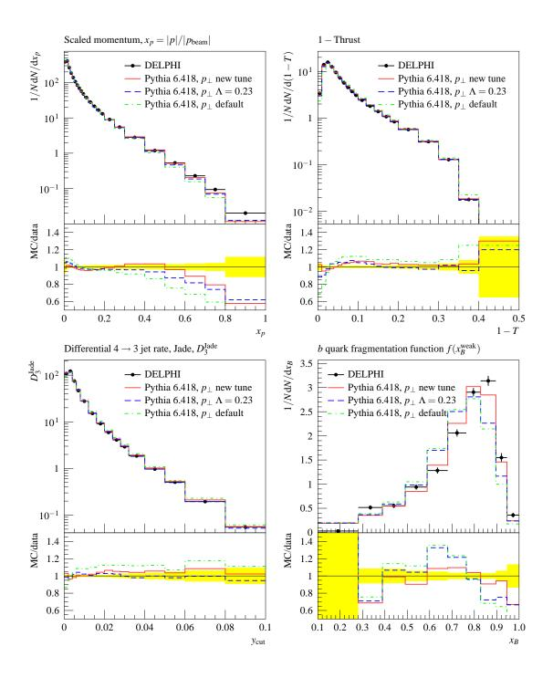
Fig. 2: Some example distributions for  $e^+e^-$  collisions using the  $p_{\perp}$ -ordered shower. The solid line shows the new tune, the dashed line is the old recommendation for using the  $p_{\perp}$ -ordered shower (i. e. changing  $\Lambda_{QCD}$  to 0.23), and the dashed-dotted line is produced by switching on the  $p_{\perp}$ -ordered shower leaving everything else at its default. The latter is the unfortunate choice made for the ATLAS-tune. The data has been published by Delphi [3,9].
