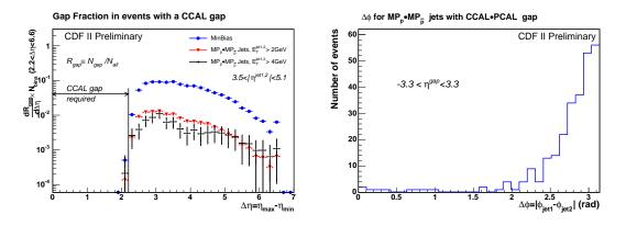
Fig. 3: Left: Event rate gap fraction defined as  $R_{gap} = N_{gap}/N_{all}$ , for minimum bias (MinBias) and MP jet events with  $E_T > 2(4)$  GeV; Right: Azimuthal angle difference  $\Delta \phi$  distribution of the two leading jets in a DD event with a central rapidity gap ( $|\eta^{gap}| < 3.3$ ).
