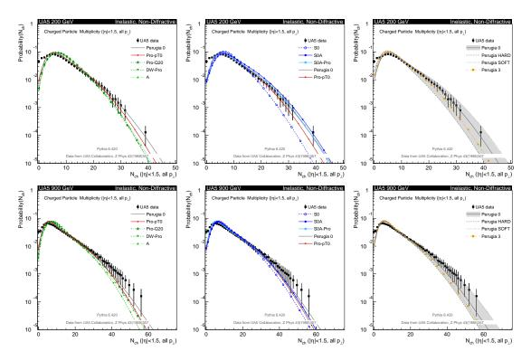
Fig. 3: Comparisons to the UA5 measurements of the charged track multiplicity in minimum-bias  $p\bar{p}$  collisions at 200 GeV (top row) and at 900 GeV (bottom row). *Left:* a representative selection of models. *Center:* different tunes of the new framework. *Right:* the range spanned by the main Perugia variations. More results can be found at [17].
