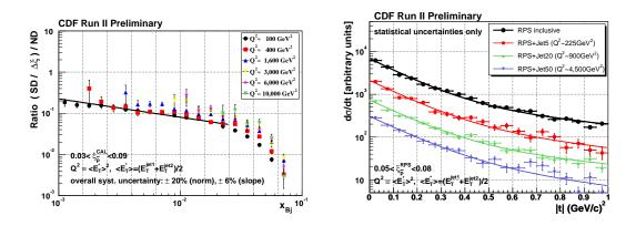
Fig. 1: Left: Ratio of diffractive to non-diffractive dijet event rates as a function of  $x_{Bj}$  (momentum fraction of struck parton in the anti-proton) for different values of  $E_T^2 \equiv Q^2$ ; Right: Measured |t|-distributions for soft and hard diffractive events.
