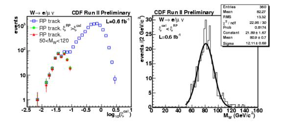
Fig. 2: Calorimeter  $\xi^{cal}$  distribution in W events with a reconstructed Roman Pot track (*left*). Due to the neutrino,  $\xi^{cal} < \xi^{RPS}$  is expected. The difference  $\xi^{RPS} - \xi^{cal}$  is used to determine the W boson mass (*right*).
