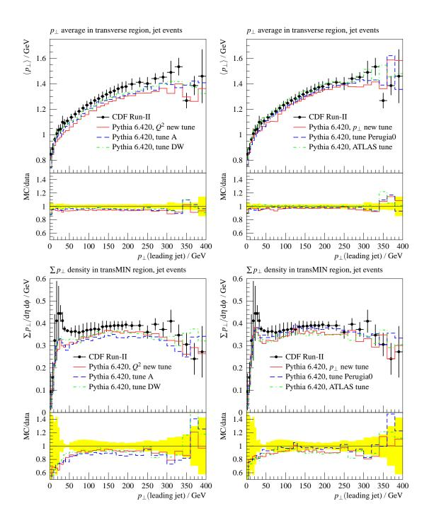
Fig. 5: These plots show the average track  $p_{\perp}$  in the transverse region (top) and the  $\sum p_{\perp}$  density in the transMIN region (bottom) in leading jet events [17]. The new model (on the right) seems do have a slight advantage over the virtuality-ordered shower with the old MPI model shown on the left, both in the turn-on hump and in overall activity.
