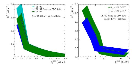
Fig. 4: Parameter space of the improved eikonal model for the Tevatron (left) and LHC (right). The solid curves impose a minimum allowed value of  $\mu^2$ , for a given value of  $p_t^{\min}$  by requiring a valid description of  $\sigma_{tot}$  and  $b_{el}$  with positive  $\sigma_{soft}^{inc}$ . The excluded regions are shaded. We used the MRST 2001 LO [19] PDFs for these plots.
