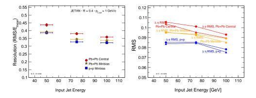
Fig. 5: <u>Left</u>: jet energy resolution versus the input jet energy of 50, 75 and  $100 \pm 5$  GeV for p + p (squares), Pb + PbMinbias (stars) and Pb + Pb Central (cirles) collisions. Right: resolutions in  $\eta$  and  $\phi$  of the jet direction.
