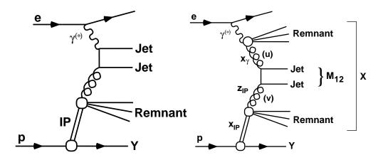
Fig. 1: Left panel: Direct-photon diagram for diffractive dijet photoproduction. Right panel: Resolved-photon diagram for the same process.
