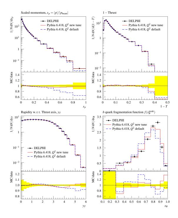
Fig. 1: Some example distributions for  $e^+e^-$  collisions using the virtuality-ordered shower. The solid line shows the new tune, the dashed line is the default. Even though the virtuality-ordered shower is well-tested and Pythia has been tuned several times, especially by the LEP collaborations, there is still room for improvement in the default settings. Note the different scale in the ratio plot of the rapidity distribution. The data in these plots has been published by Delphi [3,9].
