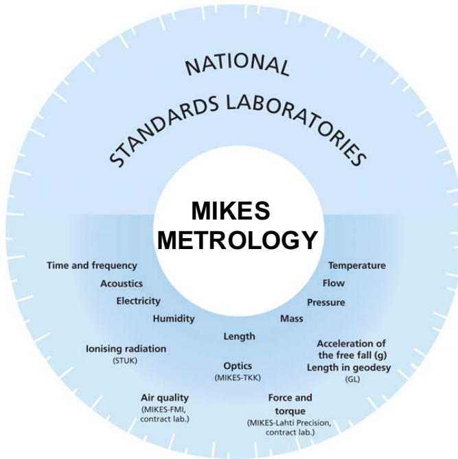
Figure 2.2. The national standards laboratories for the SI base quantities (MIKES Metrology), and those for ionization radiation (the Radiation and Nuclear Safety Authority, STUK), for optics (MIKES-TKK), for acceleration of the free fall (g) and length in geodesy (the Finnish Geodetic Institute, GL), for Force and torque (MIKES-Lahti Precision) and for Air quality (MIKES-FMI) comprise the measurement system in Finland.
