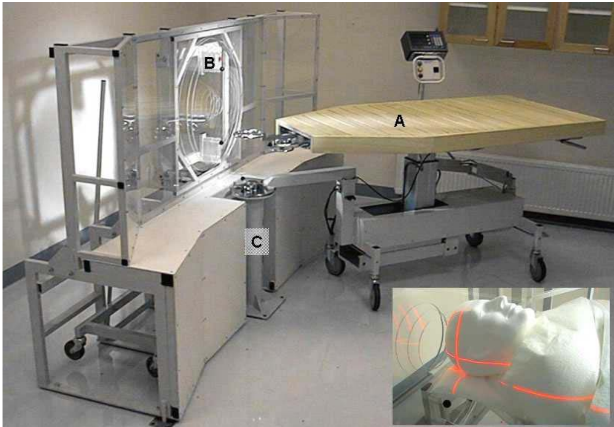
Figure 35. The treatment couch (A) and the beam simulator system (B). The couch is attached to the docking base (C). In the small image the head model has been positioned for the vertex field using vacuum cushion fixation.
