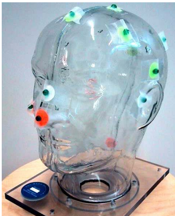
Figure 30. The antropomorphic head phantom (RSVP) with a part of the E-vitamin capsules shown on the fiducial mark locations corresponding to the transaxial, vertex and six beam entry/exit points used in the spatial accuracy study.
