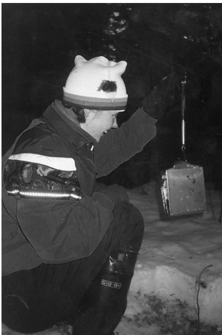
Figure 3.17. Measuring snow density by weighing a one-liter sampler.
