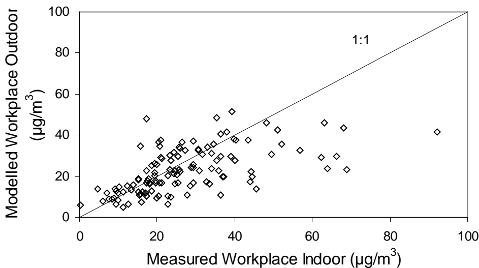
Figure 4. Modelled workplace outdoor NO 2 concentrations and measured workplace indoor NO 2 concentrations ( r^2=0.35 , n=121 ).
