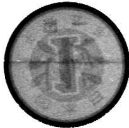
Figure 6.7. A single frame X-ray image of a Japanese coin acquired with the CdTe real time imager [82].
