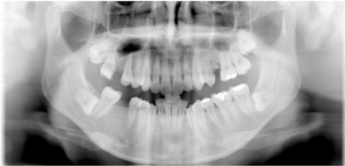
Figure 5.13. A panoramic projection image of a human skull acquired by the Ajat CMOS-CdTe panoramic camera [82].
