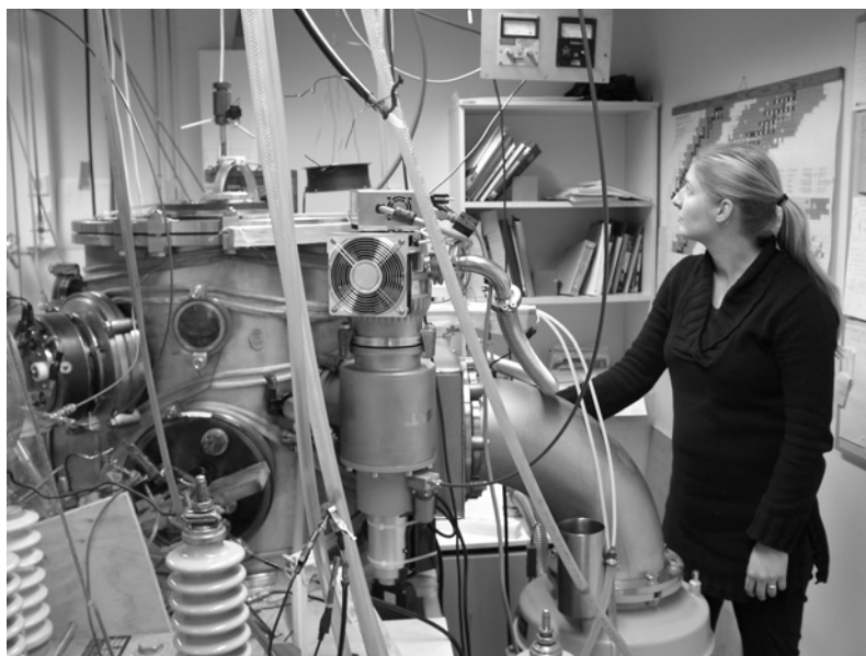
Figure 6. Plasma deposition system at the University of Helsinki Accelerator Laboratory. Attached to the vacuum chamber are: on the left is the argon sputtering unit; straight ahead the high-energy deposition unit; on the right are the turbo and oil diffusion vacuum pumps.
