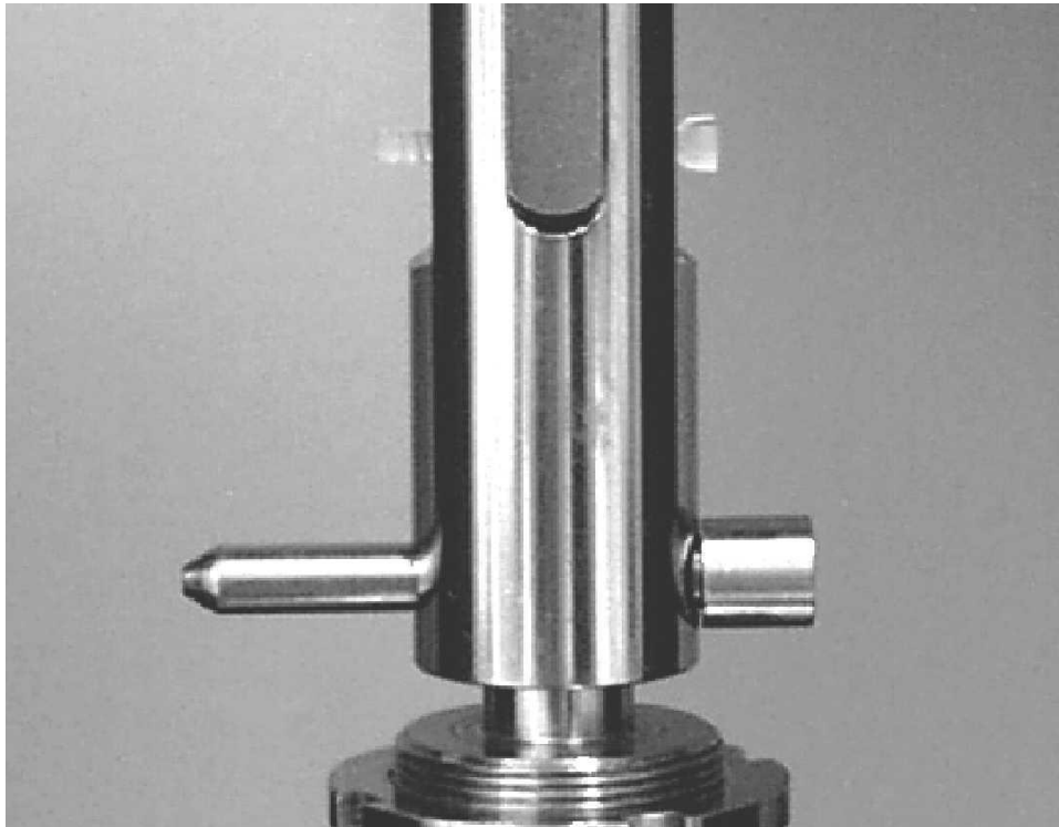
Figure 3. Two parts of the shear-strength-testing tool joined together by the implant.
