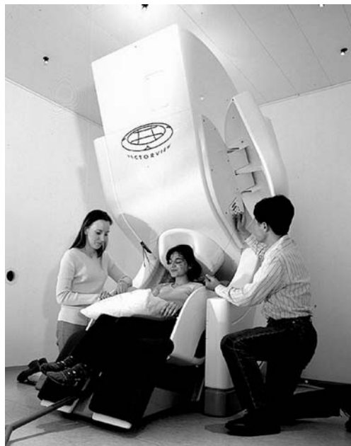
FIGURE 4 The 306-channel whole-scalp neuromagnetometer Vectorview™ (Neuromag Ltd; Helsinki). Subjects is sitting with her head supported against the bottom surface of the sensor helmet.
