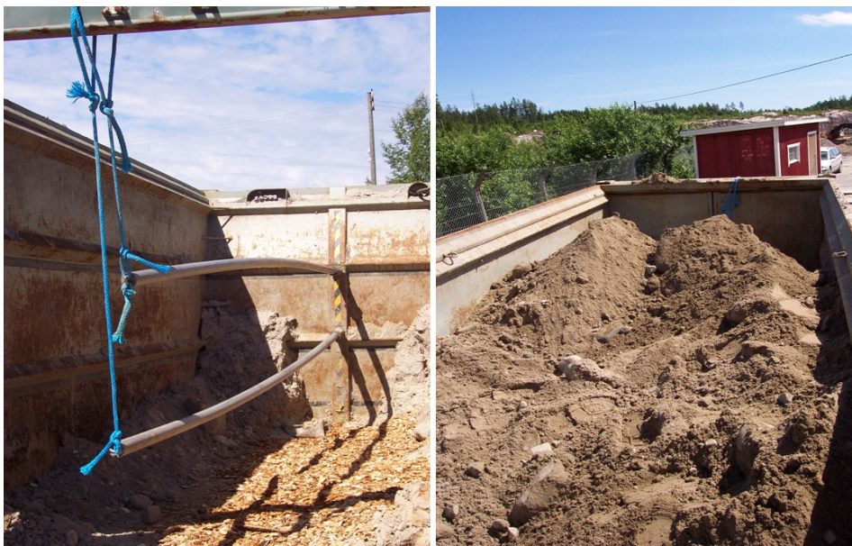
Figure 7. The BRCSoil Bioreactor used for composting the diesel oil- and lubrication oil-contaminated soil.
