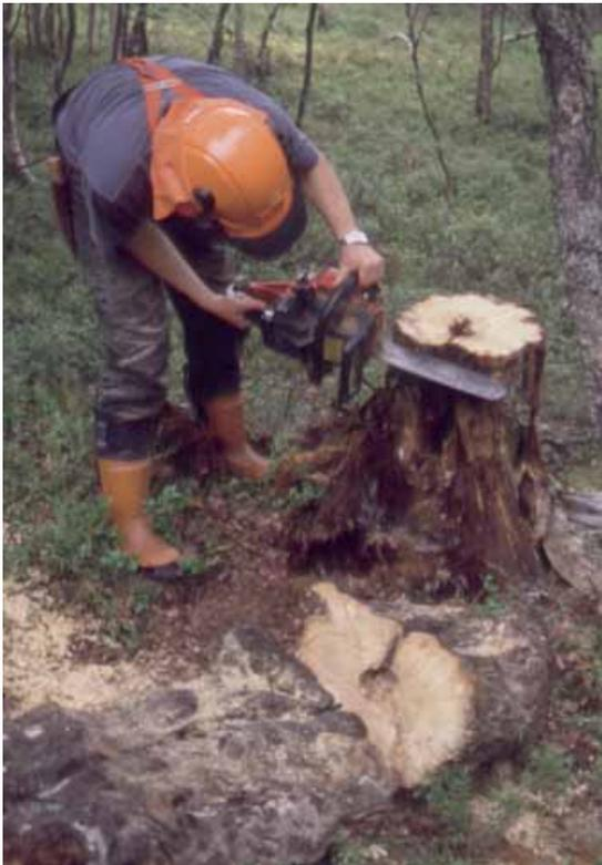
Fig. 3. Antti Lavikainen sawing a sample disk from a charred log that includes one fire scar.
