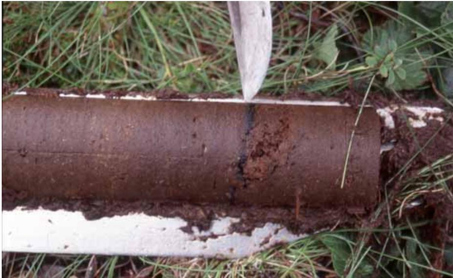
Fig. 2. A clear charcoal layer on the convex surface of a peat sample. Burning of peat and mire vegetation produces a lot of microscopic and macroscopic charcoal particles, which can be seen as a black layer of charcoal in peat. Photo: Antti Lavikainen.
