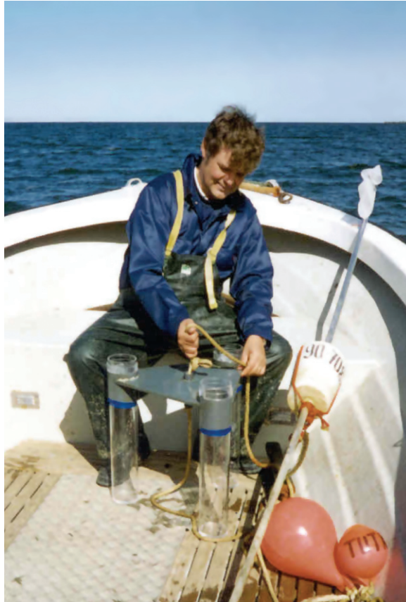
Fig. 122. A triangle-shaped sediment trap on deck.
