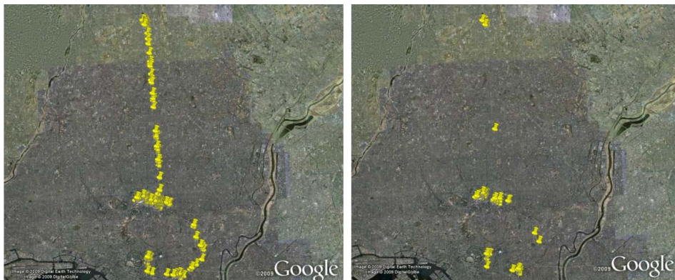
Figure 5.3: Illustration of the use of velocity information to prune data. The data in the example was collected in Tokyo, Japan. The original data set is shown on the left and the pruned data on the right. Most of the removed measurements correspond to points where the user was traveling by train.
