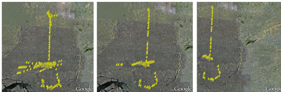
Figure 5.2: Illustrating the notions of valid and invalid points. The left-most picture contains all measurements we have collected from Tokyo, Japan. The picture indicates that there are many invalid measurements which appear as straight lines originating from a frequent location. From the picture in the middle we have removed points where less than four satellites were visible and from the right-most picture we have removed points for which the HDOP value exceeds 6.0.
