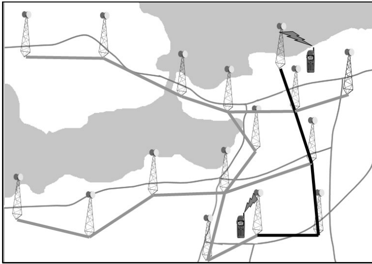
Figure 2.3: Call routing between two mobiles in the network.
