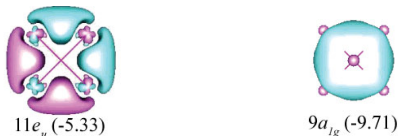
Figure 4.6: The HOMO (left) and HOMO-1 (right) molecular orbitals of \text{Li}_2\text{Cu}_4 calculated at the HF SCF/TZVPP level using the MP2/TZVPP molecular structure. The orbitals are viewed along the C_4 axis. The orbital energies (in eV) are given within parentheses. The pictures have been made using gOpenMol [137].
