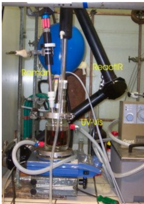
Figure 34. The set-up to perform UV-Vis, Raman and ATR-IR spectroscopic measurements simultaneously.
