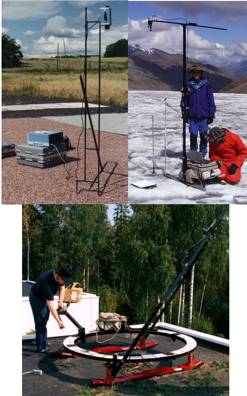
Figure 2. Some older manual goniometer models that were developed and used at Finnish Geodetic Institute. Top left picture shows the first model, bottom one shows model 3 and top right one model 4. The operation principle of model 4 is quite similar to our current device, model 5 a.k.a. FiGIFiGo. (Pictures by Jouni Peltoniemi)
