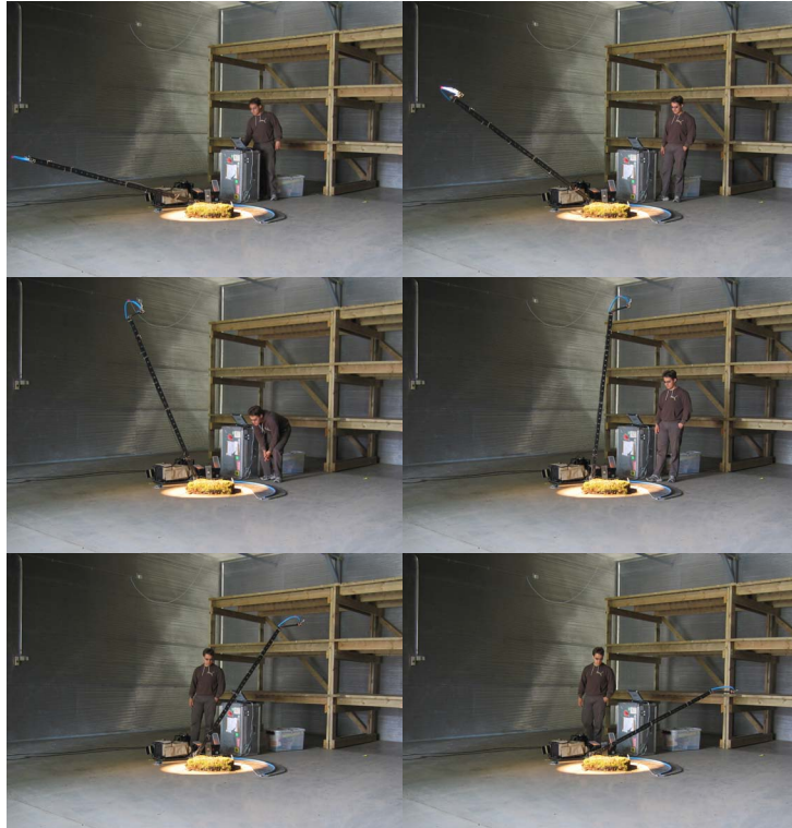
Figure 8. FiGIFiGo in operation. FiGIFiGo measures automatically the reflected spectrum from a series of beforehand-defined zenith angles. Typically measurements are done at zenith angles from -70^{\circ} to +70^{\circ} between 2.5^{\circ} or 5^{\circ} interval. Measurement of one such arch takes 60-120 seconds depending on the interval and integration time. The filmstrip was photographed in laboratory at METLA research station in Suonenjoki.
