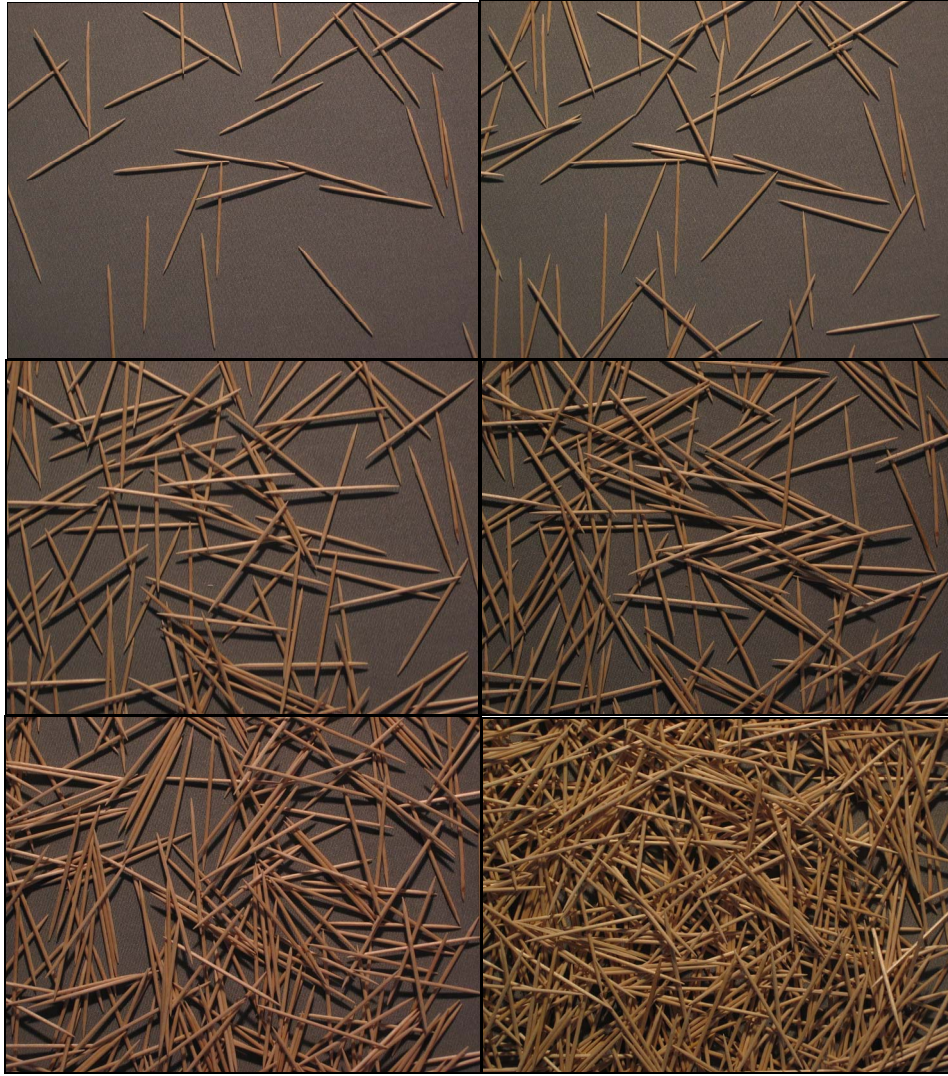
Figure 13. Nadir photographs of samples with 12 (top left), 25, 50, 75, 100, and 225 (bottom right) grams of bright cocktailpicks scattered over area.
