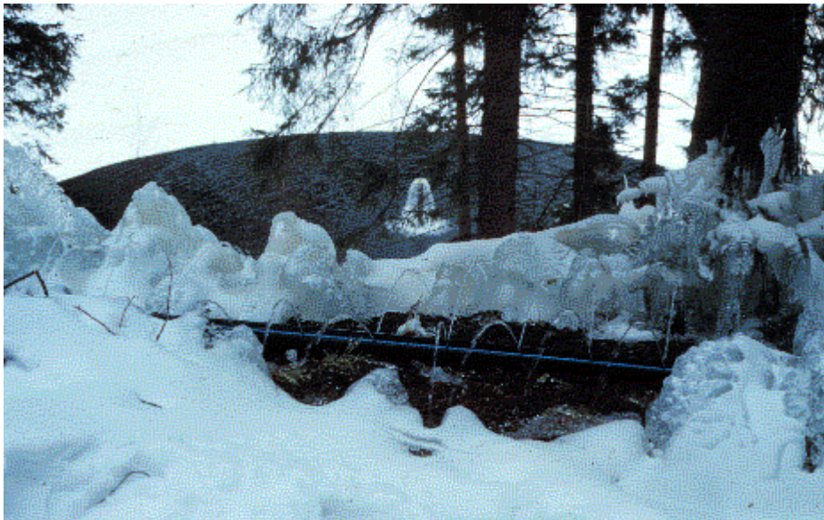
Figure 4. The Ahvenisto sprinkling infiltration experiment: (a) continuous infiltration during the summertime, (b) continuous infiltration during the wintertime.
