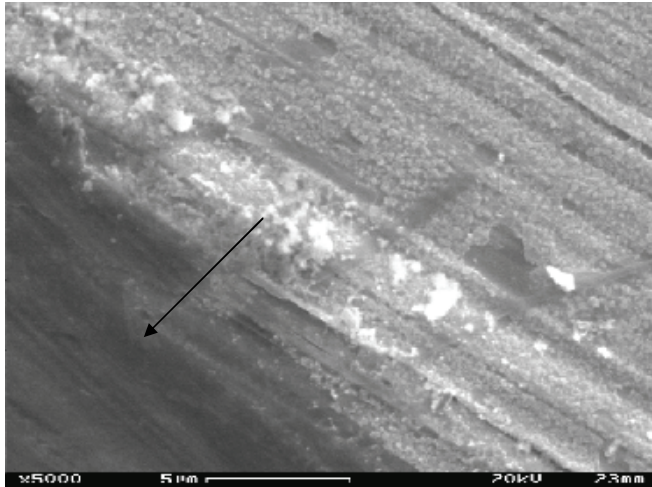
Figure 9: Organic layer deposited within one day on a coupon immersed in the white water channel in a paper mill using recycled fiber. A manual scratch (arrow) uncovered the clean steel surface (SEM-micrograph, magnification x5000).
