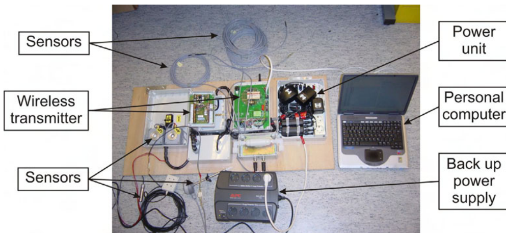
Figure 7. Components of the wireless monitoring and measurement system.
