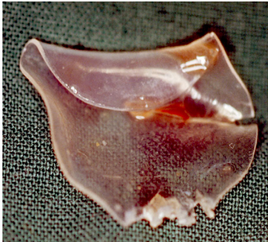
Figure 7. The SR PLDLA 96/4 implants were deformed after only 3 months without any macroscopic signs of degradation.
