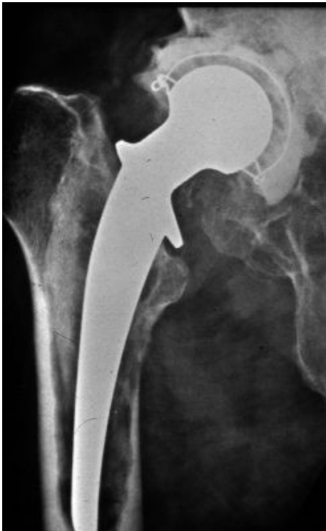
Figure 1. X-ray picture from a loose THR prosthesis. Metal wire surrounds the ultra-high molecular weight polyethylene acetabular cup, which is not otherwise visible in the picture. Radio-opaque agents make PMMA cement around the cup visible. Dark areas in the femur indicate osteolysis.
