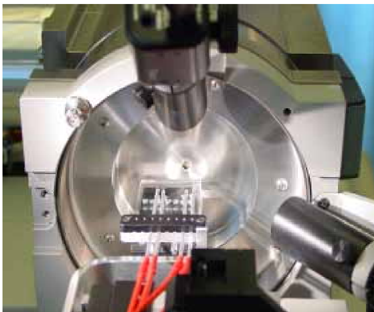
Figure 14. A modified platform for aligning a PDMS chip toward the MS inlet. ESI voltage was applied through platinum electrode wires on the sample reservoir on the chip.
