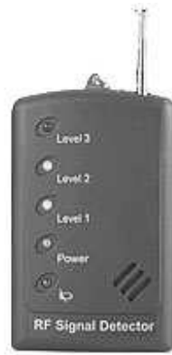
Figure 10.4: An example of a detector for RF-signals. (Figure from http://ucables.com/ref/RF-DETECT1/ .)
