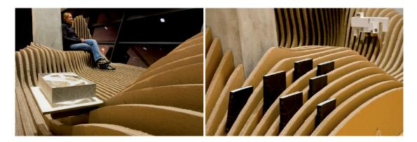
By focussing the water-jet to a diameter of 0,02mm and a pressure of 3000 bar the fluid cutting medium has no negative effect on the cardboard material.
