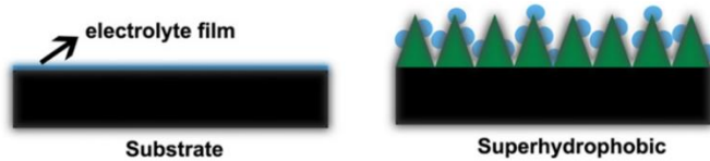
Figure 9: Models for corrosion resistance of superhydrophobic surfaces (a) in corrosive solution; (b) in humid air [171].
