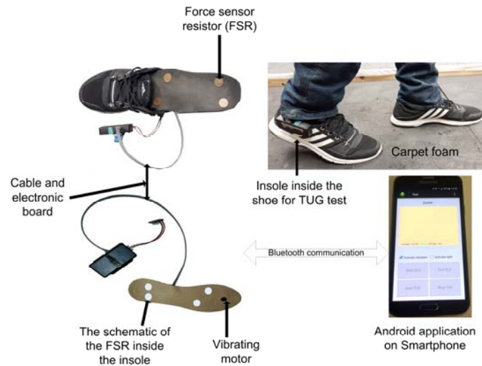
Figure 1. The ACHILE system (two types of enactive insole and Android application)
