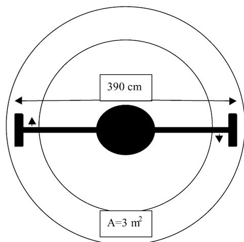
Fig. 1. Schematic picture of the axle system with direction of rotation and the distance between the tyres. The area of the driving space is also shown.
