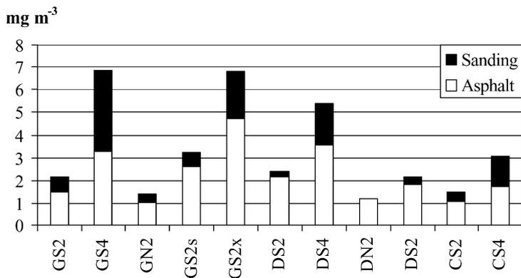
Fig. 5. The average shares of the PM<sub>10</sub> from the asphalt and the traction sand. For abbreviations see Table 2, tyre.
