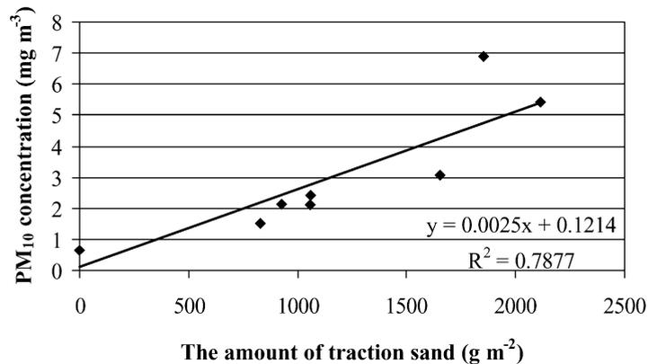
Fig. 3. The correlation between ambient  $PM_{10}$  concentrations and the amount of traction sand used for the studded tyres.
