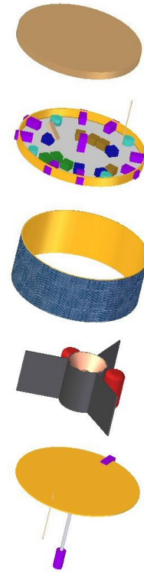
Figure 10: The main hardware parts of the WARP spacecraft are the cylindrical shell serving as the structural body with two faceplates, the instrument platform and a thermal protection layer. The instrument platform can also be realized as two smaller platforms to accommodate the key system devices in the vicinity of each other.
