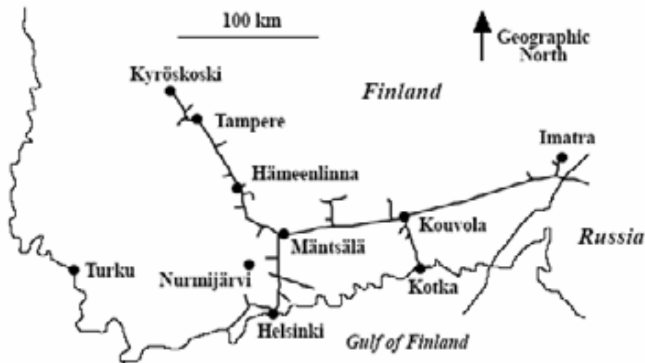
Figure 4-4 Finnish natural gas pipeline network. GIC measurements with a magnetometer are performed at Mäntsälä (Pulkkinen et al., 2001b). The Nurmijärvi Geophysical Observatory is located about 30 km to the southwest from Mäntsälä.
