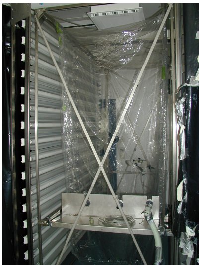
Figure 3.3. The indoor smog chamber at the Laboratory for Atmospheric Physics and Chemistry, University of Kuopio.
