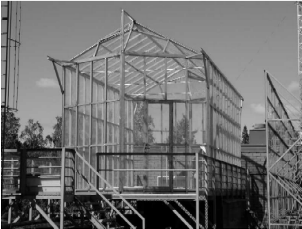
Figure 3.2. The outdoor environmental chamber at the Laboratory for Atmospheric Physics and Chemistry, University of Kuopio. The long walls of the chamber are in NW-SE orientation, NW end near the building behind the chamber. On the right is a wind shield.
