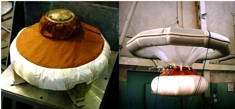
Figure 11: Engineering model of the MetNet Lander being exposed to a set of mechanical tests.
