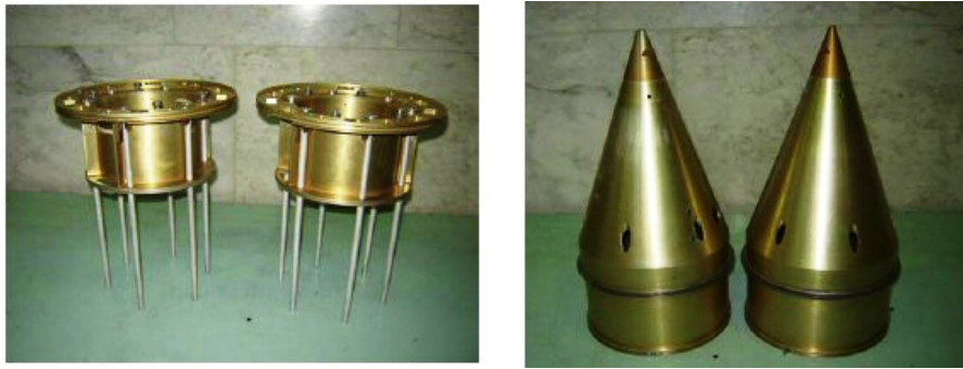
Figure 13: Two sets of Flight Unit payload bays are shown above with the end cone of the two MetNet Lander Flight Units also depicted in the preceding figure 12. The payload compartment will slide downwards during the impact and some of the mechanical energy is consumed by the metallic rods.
