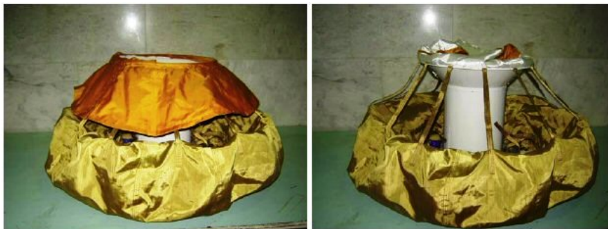
Figure 12: Two complete Flight Units of the MetNet Lander with all the entry, descent and landing systems have been manufactured. They will be used in the MetNet Mars Precursor Mission slated for launch in 2009/2011.
