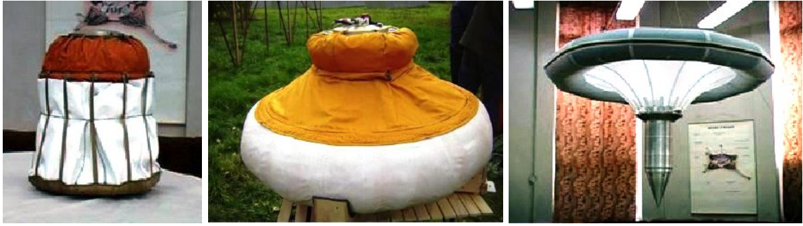
Figure 9: The left image shows the MetNet configured for descending. The middle image shows a flight test version with the heat shield fully inflated. The right shows the MetNet configured for landing. The circular tube-like structure above the MetNet station is a second stage inflatable for deceleration after the hypersonic entry phase.
