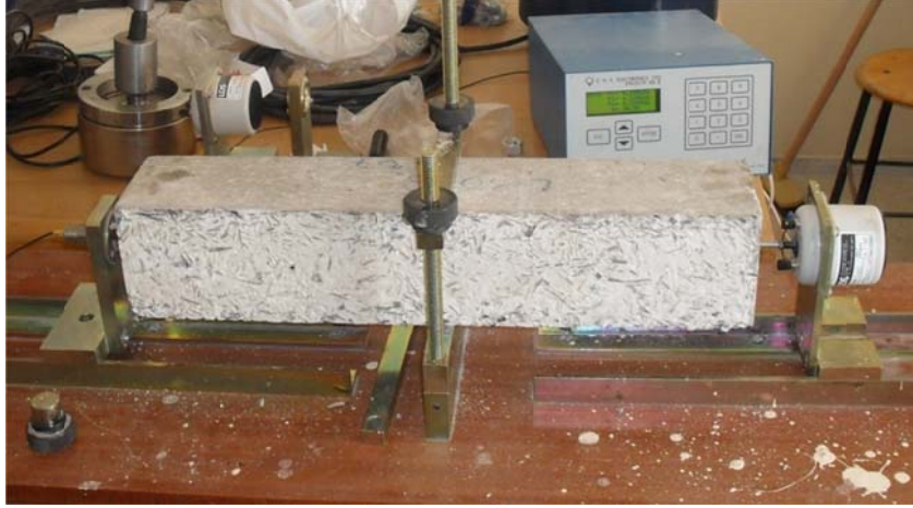
Fig. 2 Resonance frequency measurement on concrete
