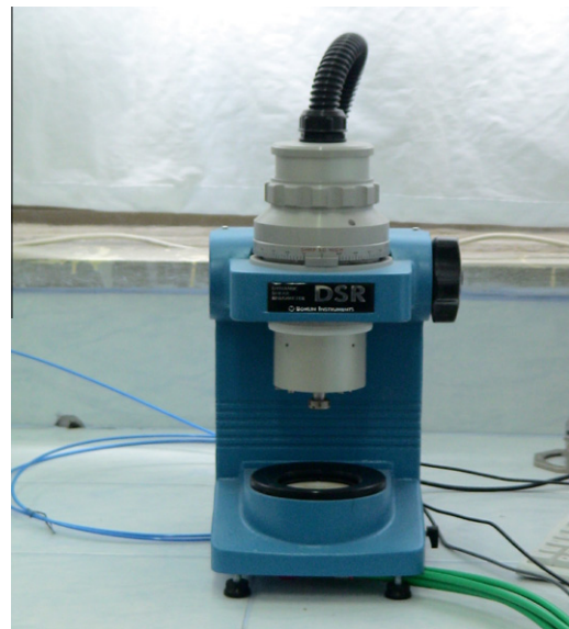
Fig. 2. DSR test machine.
