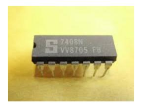
Figure 4-7: 7408 chip, notch indicates top of chip.
