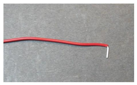
Figure 3-5: A stripped wire
