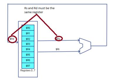
Figure 1-7: 2-address architecture
