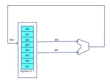
Figure 1-6: 3-address architecture
