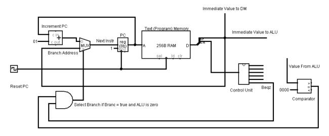
Figure 5-6: CPU - Execution Path Subsection
