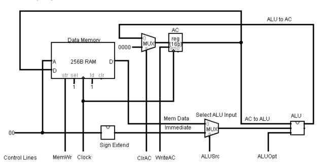
Figure 5-5: CPU - Arithmetic Subsection
