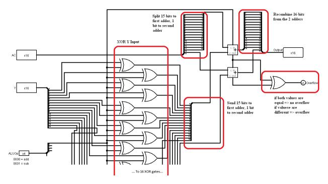
Figure 5-4: Adder/Subtracter with overflow
