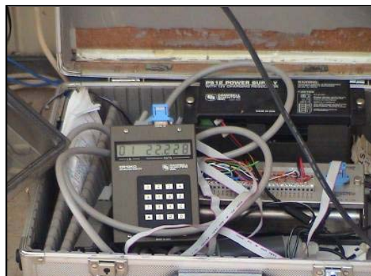
Fig. 3. a) thermocouples; b) datalogger; c) digital thermometer.
