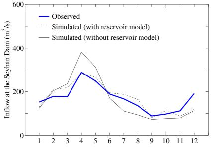
Fig.5 Simulated hydrograph at the Seyhan Dam.
