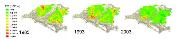
Fig. 10 Electrical conductivity of shallow water table in July in the LSIP.
