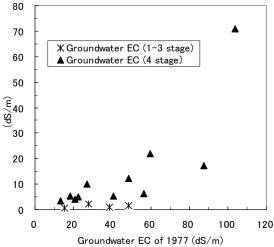
**Fig.7.** Relationship between groundwater EC in 1977 and 2005-2006
