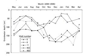
**Fig.5.** Fluctuation in the groundwater depth along transects A and B
