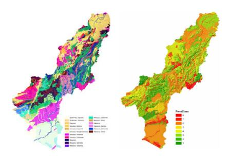
Figure 4.2 Simplified geological and permeability class maps of the Seyhan River Basin
