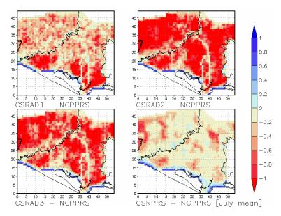
**Fig.7** Comparison of water table level between present and different adaptation scenarios (The case of CCSR runs in july average, scenario 1: top left, scenario 2: top right, scenario 3: bottom left, present landuse: bottom right ).
