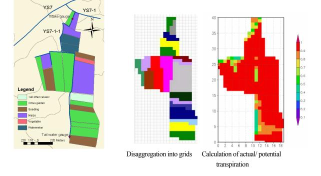
**Fig. 4** Land use in command area of YS7-1-1, disaggregation into grids, and the example of grid calculation by the IMPAM.
