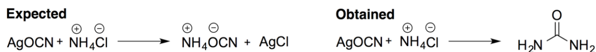
Figure 1. Wöhler's synthesis of urea, which represents a landmark achievement in organic synthesis and biological chemistry.
