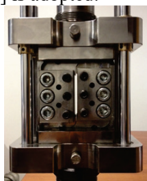
Figure 1. Simple shear device for AHSS
