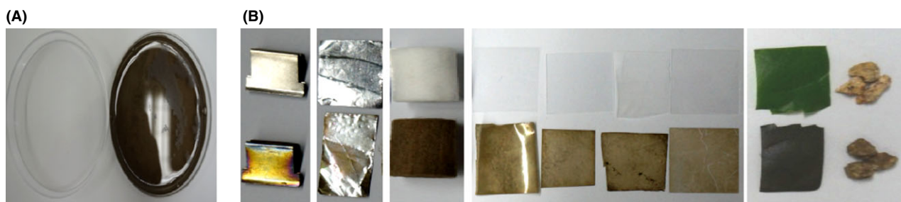
Fig. 1. One-pot modification of solid surfaces through in vitro laccase-catalysed polymerization of 2,7-DHN.
