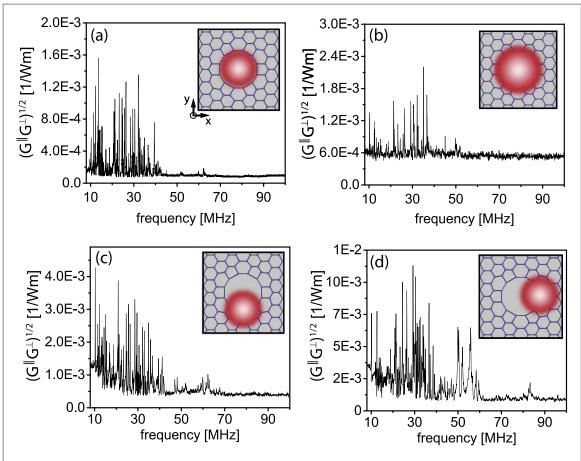
**Figure 8.** Misaligned Brillouin gain measurements for the (a) ideally coupled case and with the fiber offset by (b) 50  $\mu$ m in the z-direction (i.e. defocused via motion towards the lens), (c) 5  $\mu$ m in the y-direction (vertical), and (d) 5  $\mu$ m in the x-direction (horizontal). The insets in are iconic representations of the implemented offset.
