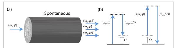
Figure 3. Hollow-core fiber with (a) input and output fields and (b) respective energy-level diagram for a spontaneous Stokes and anti-Stokes scattering process (polarized or depolarized GAWBS).
