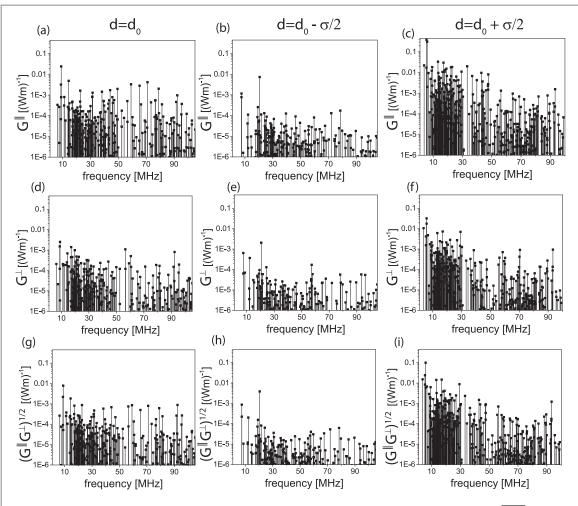
**Figure A1.** Simulated forward Brillouin gain for the three distinct gain coefficients: (a)–(c)  $G^{\parallel}$ , (d)–(f)  $G^{\perp}$ , and (g)–(i)  $\sqrt{G^{\parallel}G^{\perp}}$ . The geometry is specified by the column label and is defined as in figure 7.
