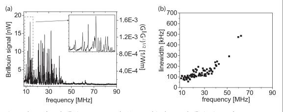
**Figure 5.** Ph-FWM forward Brillouin measurement results. (a) Measured signal power and Brillouin gain versus frequency. Inset: an enhanced view of the first few resonances. (b) Full-width at half-maximum linewidths of the identifiable resonances from (a).
