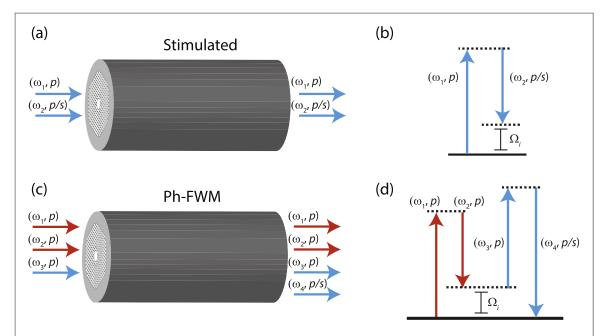
**Figure 2.** Hollow-core fiber with input and output fields and respective energy-level diagram for (a), (b) stimulated Stokes scattering process and (c), (d) the phonon mediated four-wave mixing process described in this work (both inter- or intra-polarized versions). Each frequency is indicated with a number and a polarization in parenthesis. Note that (c), (d) depicts one specific anti-Stokes interaction; the corresponding Stokes process occurs simultaneously.
