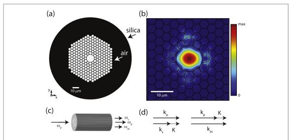
**Figure 1.** Hollow-core fiber (a) cross section and (b) near field intensity profile of the fundamental optical mode obtained by the simulation methods described in section 5. (c) Brillouin frequencies of interest in the HC-PBF, indicated as inputs and outputs. (d) Phase matching condition for the Stokes and anti-Stokes processes, respectively.
