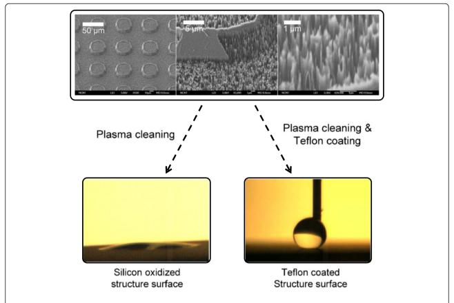
**Figure 1 SEM image and apparent static contact angle.** SEM image of the fabricated structured surface and apparent static contact angle on oxidized silicon and Teflon-coated nano/microstructures.
