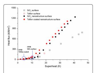
Figure 2 Comparison of boiling curve on each of the different heating surface conditions.
