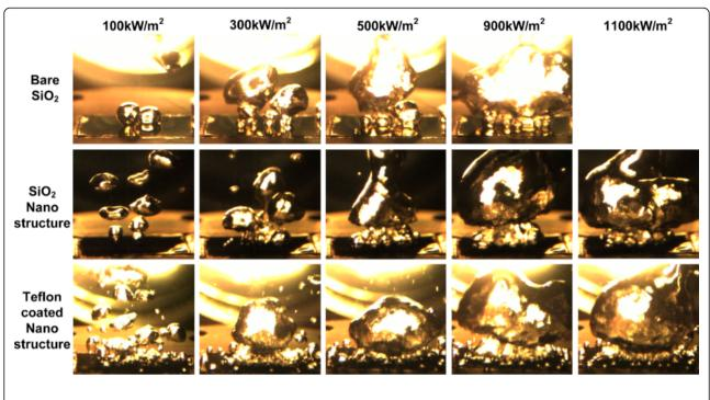
Figure 5 Bubble dynamics on each of the different heating surface conditions at different heat flux conditions.
