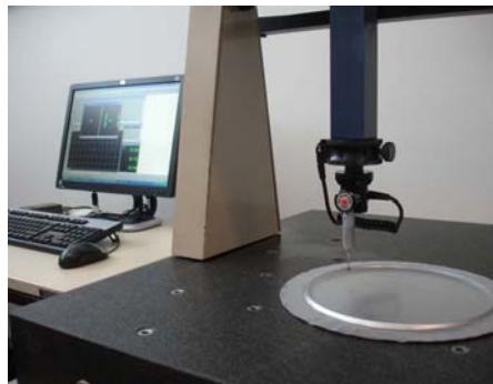
FIGURE 12. CMM Measurement of bulge specimens for different bulge pressures.
