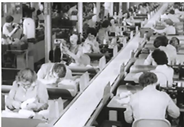
Figure 2-7. The newly designed closing shop. Note the automated conveyor belt for moving work to and from each work station. 170
