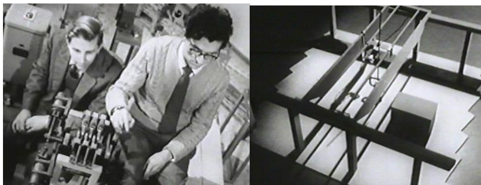
Figure 2-9. Laboratory mock-up of crane controls and rapid prototyping to determine prime cab position on the gantry.
