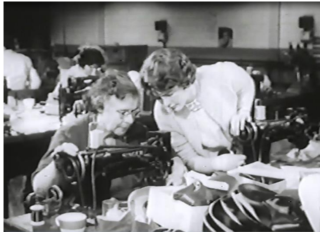
Figure 2-6. Slowing the sewing machine using hand pressure on the balance wheel. 167
