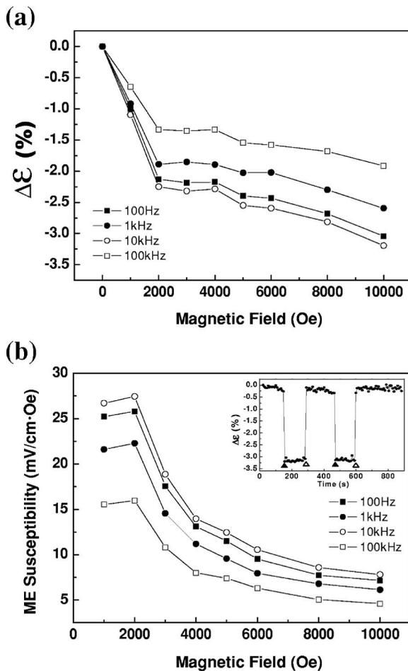
FIG. 3. ME coupling characteristics of the 450-nm-thick PZT/NZFO multilayer consisting of 11 alternating layers. (a) Percent change in the real part of dielectric permittivity at various measuring ac electric-field frequencies. (b) Longitudinal ME susceptibility plotted as a function of  $\Delta H_3$ .
