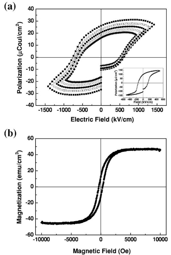
FIG. 2. (a)  $P$ - $E$  hysteresis loops obtained at  $1 \text{ kHz}$  and (b)  $M$ - $H$  hysteresis curve of the PZT/NZFO multilayer structure consisting of 11 alternating layers.
