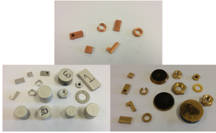
Fig. 2. Test samples. Sixteen Aluminium (left), fourteen brass (right), and six copper pieces (top).
