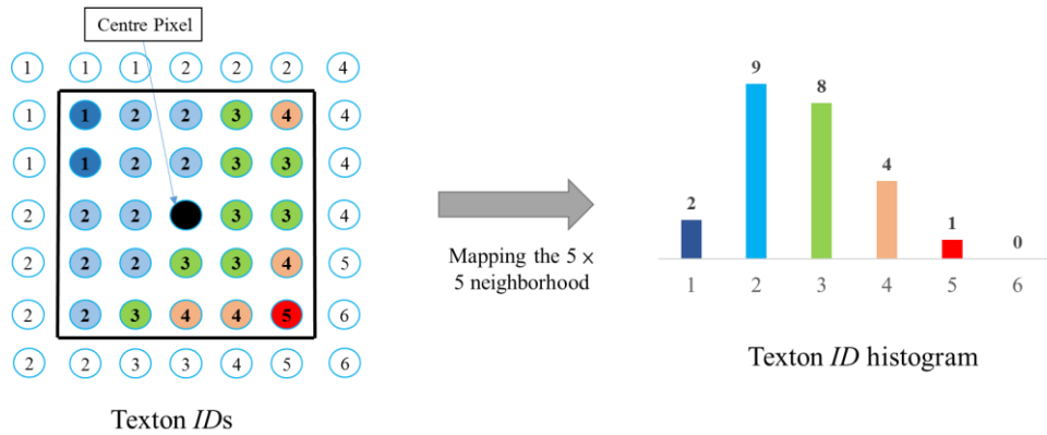
Figure 6-9 The connectivity of the adjacent pixels from the histogram of the texton IDs in a 5 \times 5 neighbourhood of the centre pixel. The texton clusters are integers in the range [1, 6]. The texton IDs outside the neighbourhood are not counted. This is a simplified example to illustrate the procedure of texton histogram feature extraction from the pixel neighbourhood. The texton histogram values are zero for IDs from 6 to 16 in this example.
