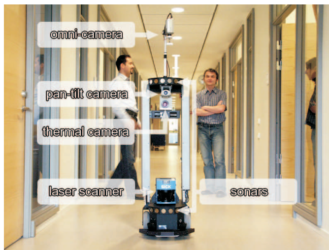
Fig. 1. Robotic platform for security guard with sensors marked. The laser range scanner and the omni-directional camera is used to build a 3D model of the robot's operation environment.
